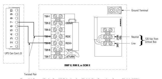
Figure 5-8. Remote Monitor Panel II, Relay Interface Module II, or Supervisory Contact Module II Wiring
